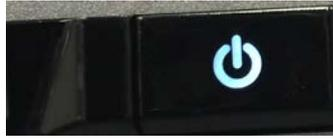
Push the power button to power on the display. This will also power on the Windows computer that is built into the display.
